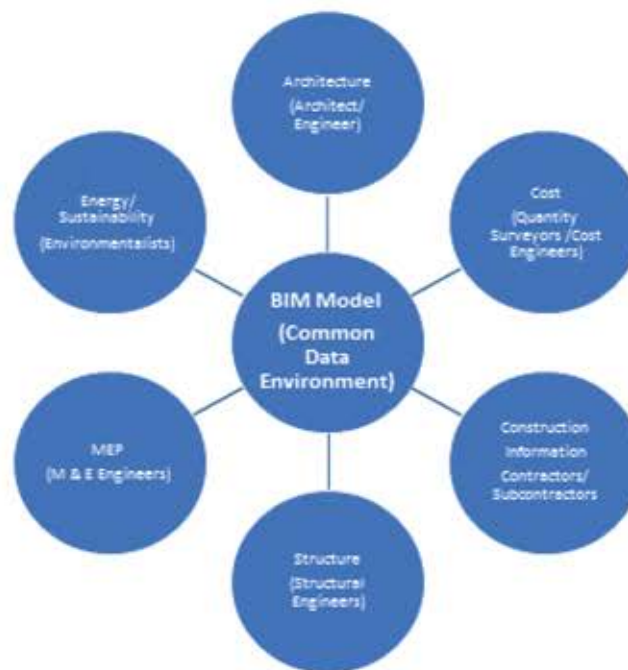
Figure 1: Development of BIM Model and Interaction of Stakeholders
