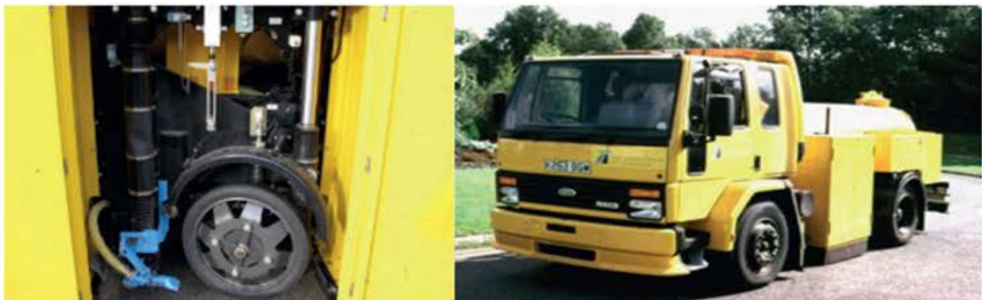
Figure 4: Sideways Force Coefficient Routine Investigation Machine used for SFC survey at network level in the UK (Source: WDM, UK)
