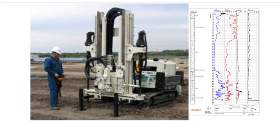
Figure 10: Field testing (Cone penetration testing) (Source:Website-3: sfc.com.sa)
