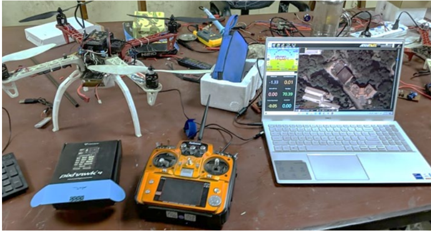
Figure 3. The laboratory workbench shows the prototype quadcopter drone, remote controller, telemetry data receiving laptop and associated system parts and accessories
