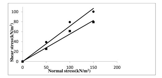
*Figure 4: Failure envelopes of river sand and FAPS specimens*
