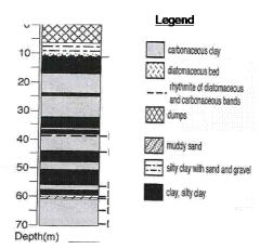
*Figure 4 Typical soil profile along the Kathmandu line (E-W direction) (Sakai et. al, 2001)*
