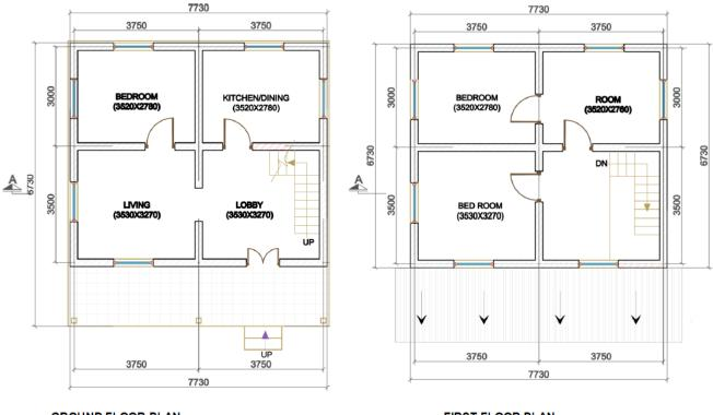
GROUND FLOOR PLAN FLOOR AREA: 52.02SQ.M FIRST FLOOR PLAN FLOOR AREA: 52.02SQ.M
