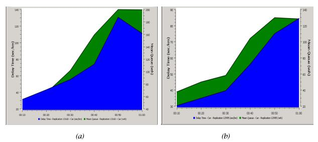
*Figure 7: Delay and queue results for 15-minute time period for (a) existing method (b) proposed method of signal control*
