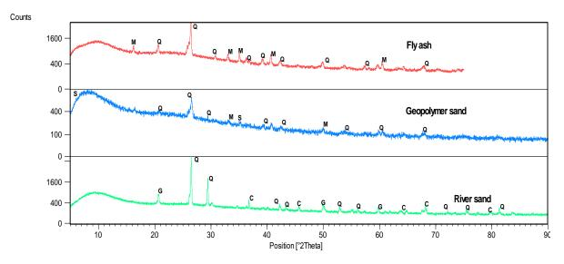
*Figure3: XRD pattern of fly ash, FAPS and river sand M* = *Mullite (Aluminum silicate) and Q* = *Quartz, G*=*Gibbsite, C*=*Calcite*
