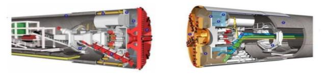
Figure 8(a) EPB TBM
