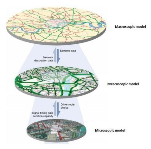
Figure 2: Transport Modelling Hierarchy (Adapted from TfL, 2010)
