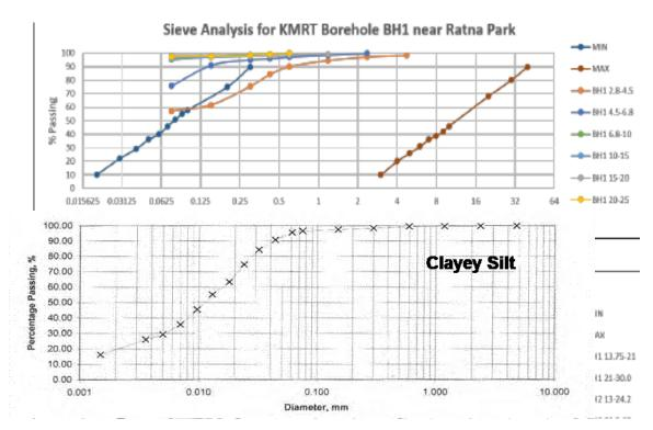
Figure 5 Particle size distribution of Kathmandu soil at central, south, east and west site
