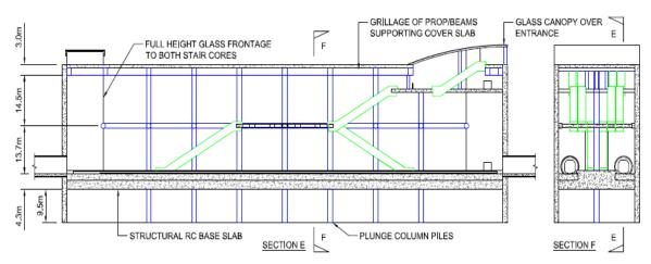
Figure 13 Typical box type local underground station for New Baneshwor station
