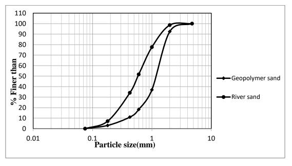
Figure 2: Grain size distribution of river-sand and FAPS specimens
