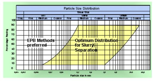
*Figure 7 Tunnelling machine selection method based on Particle Size Distribution (Slocombe, 2017)*
