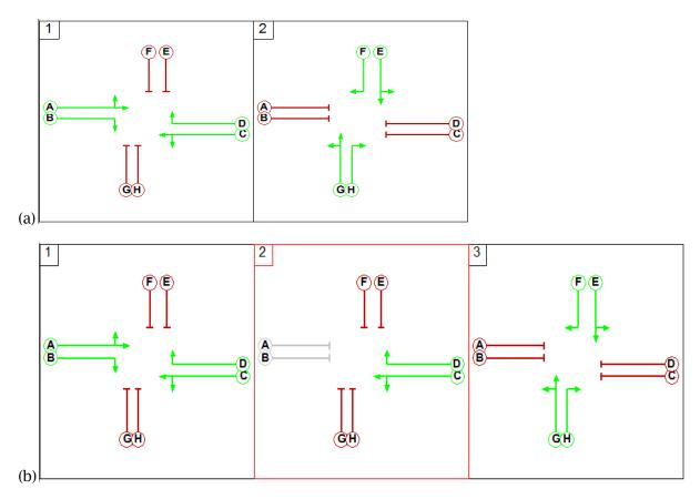
Figure 5: (a) existing method (b) proposed method of signal control
