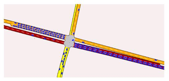
Figure 6: Vehicle queuing at the junction at the end of the simulation
