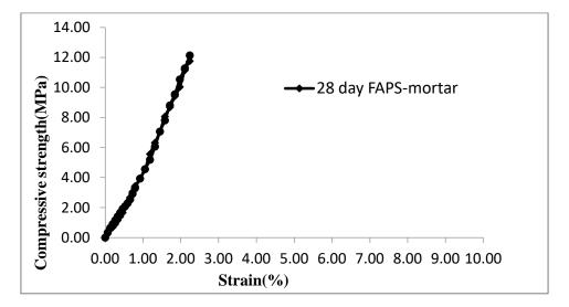
Figure 6: Stress-strain curves of mortar specimens
