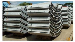
Figure 9(b) Precast concrete segment lining
