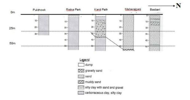
*Figure 3 Typical soil profile along the Patan line (N-S direction)*
