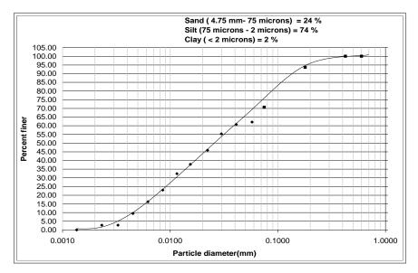
Figure 1: Particle size distribution of fly ash
