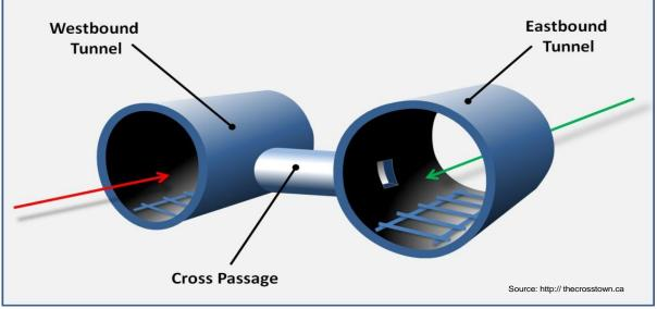
Figure 10 Cross passage tunnel
