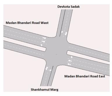
Figure 4: Junction layout of New Baneshwor Junction
